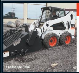
The S175 is the beginning of the vertical lift path line up. This entry level machine is very maneuverable in tight areas, has ample auxiliary hydraulic flow to run the majority of attachments, and has excellent reach at the top of its lift cycle for loading trucks or pallet fork applications.
