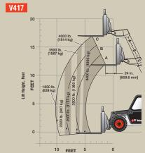
${}^{\star}\text{Rated Load Capacity can change depending on which approved attachment is used.}$
